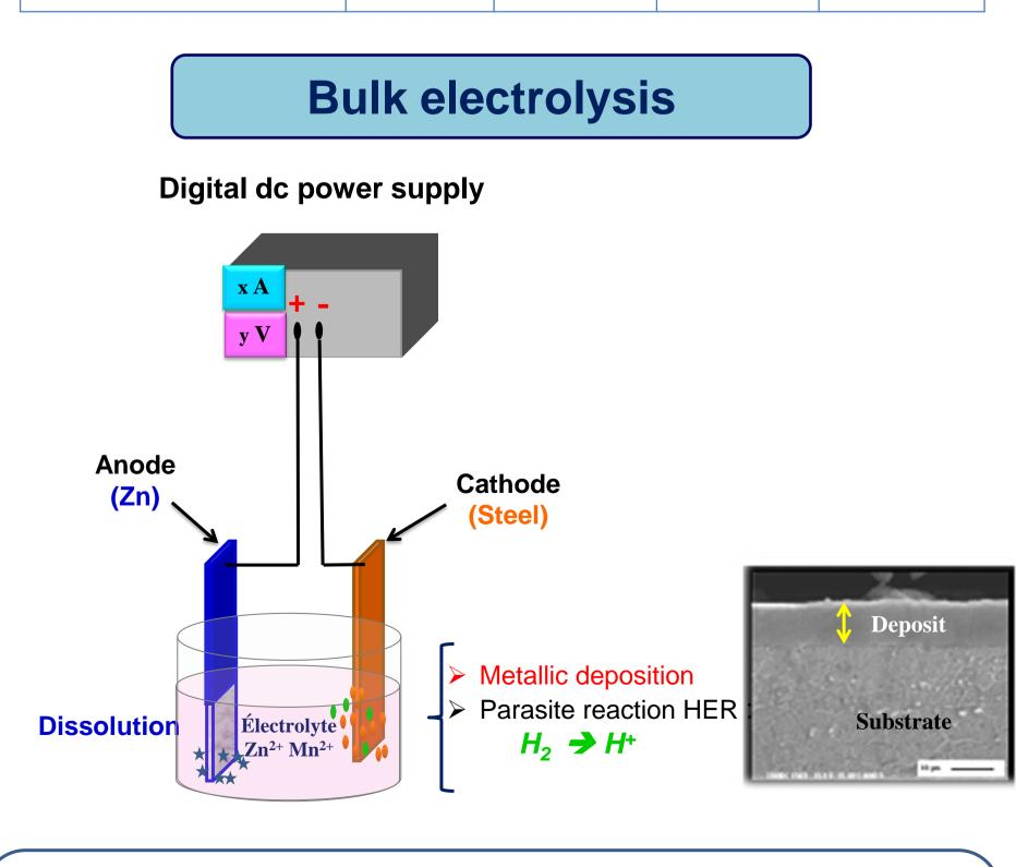
Galvanostatic experiments were carried out from the working electrolyte
